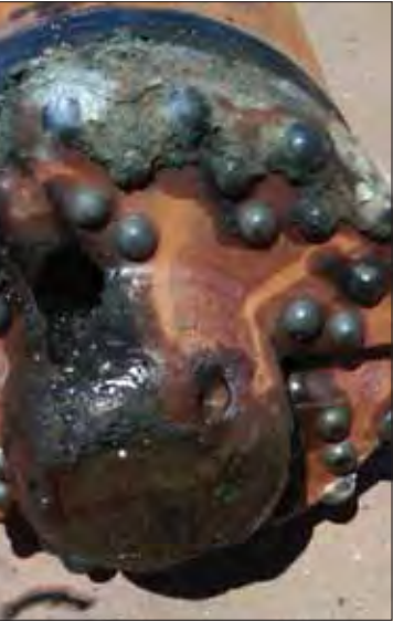
♦♦♦ The two Center Rock drills that made it all the way down: 5 and half inch CR120 bit hole opener (top) and 26 inch LP drill (bottom)
