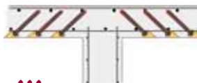
◆◆◆ Shear reinforcement rebars are installed at a 45° angle to increase shear capacity at column/slab interfaces of concrete structures
