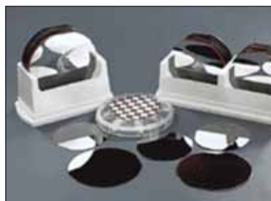
*** Fig 6 Super polishing of silicon on sapphire for LED applications
