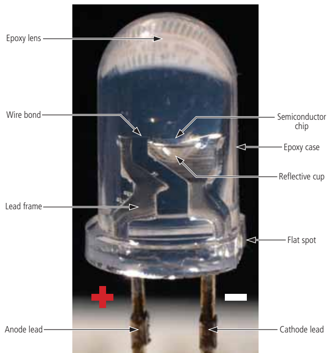
*** Fig 7 An ultraviolet LED – a more highly polished ceramic substrate surface will emit more light for the same energy input
