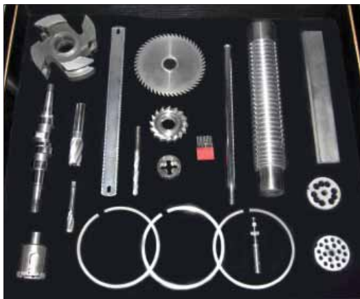
◆◆◆ Fig 4 A selection of parts that have been plated with nanodiamond for practical applications
